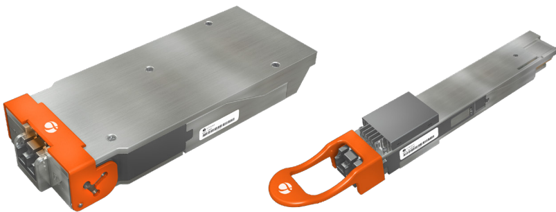
Figure 1: ICE-X intelligent coherent pluggables in CFP2 and QSFP-DD form factors
